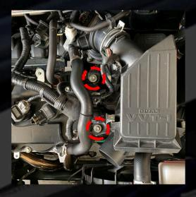
4. Unpin the cable pin beside the air intake box.
