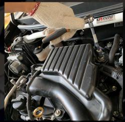
2. Remove the clip by using hand plier.
