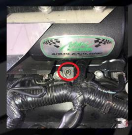
21. Plugged in the air filter, tighten it, then place on the top cover & make sure the heat shield are aligned then tighen the M13 bolts on.
