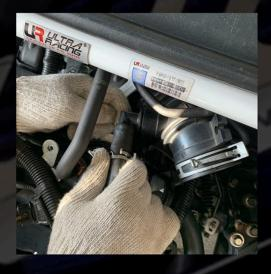
11. Remove the clip by using hand plier.
