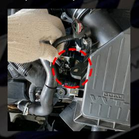
5. Remove the stated sensor screws by using philip socket with hander.
