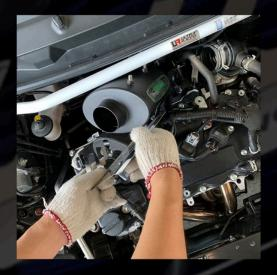
19. Carefully attach the sensor into the rampipe sensor adapter and screw it with provided Allen m3 screw. (\*\*\*make sure the Sensor are fully inserted into the adapter)
