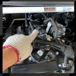
13. Remove the 10mm screw from steel bracket which behind the engine.
